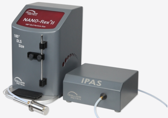
NANO-flex® II with IPAS extension for inline measurements
